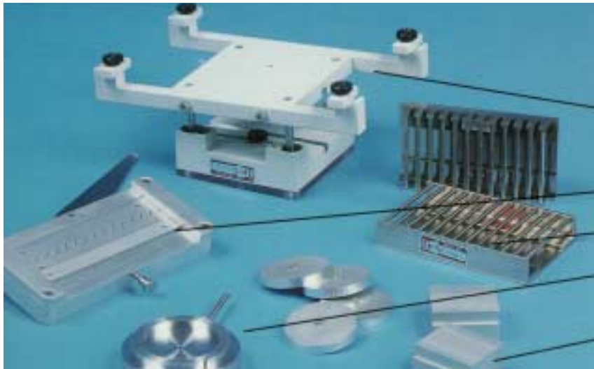
Edge compression fixture (Weyerhaeuser type)
