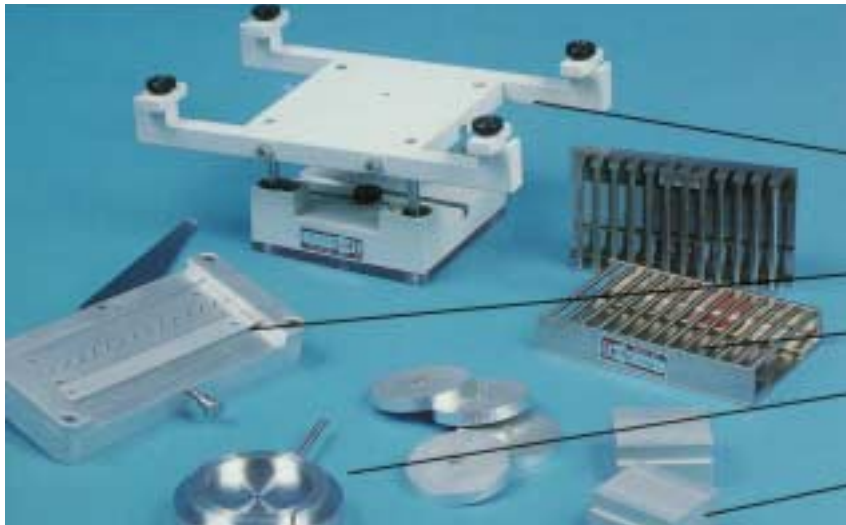
Edge compression fixture (Weyerhaeuser type)
