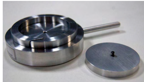
▲ RCT- Ring Crush holder with disks 17-11-13
