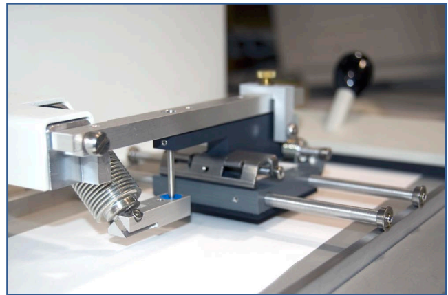
▲ Elevator System automatically raises and lowers sled
