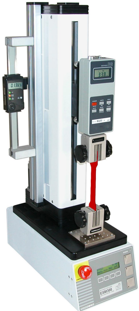
▲ The Force Test Stand is shown in a typical tensile testing application, with Series BG digital force gauge, digital travel display, and parallel jaw grips
