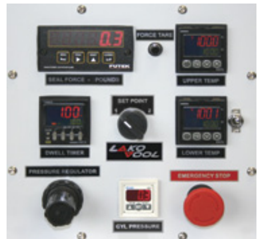
(above) All aspects of the process are controllable on the front panel using digital inputs and displays.
